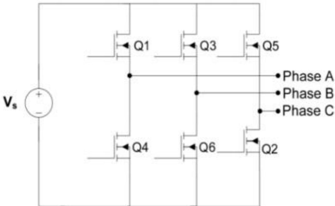
Figure 1: basic IGBT inverter circuit
